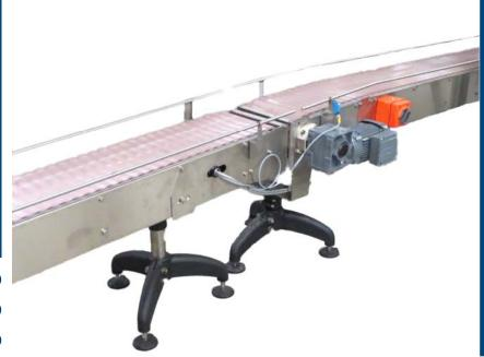
Our slat chain conveyor is mostly common in bottling and canning plants but many other applications also exist. The conveyor is made from all non-corrosive materials to make it fully wash down. SLT benefits from using standard type slat chain.
